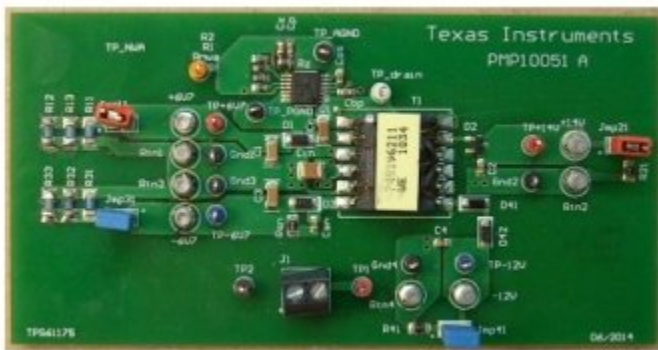
Figure 14: TI-TPS61175 Voltage Booster
